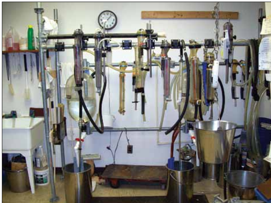
The DHI system allows use of many types of portable meters in its programs. Portable meters are calibrated using an approved water test at one of 39 U.S. QCS-certified meter centers by a QCS-certified meter technician at least once every 12 months.
